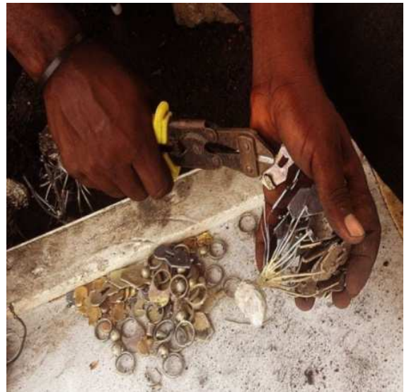
Figure 18. Cutting away sprues & gate.
