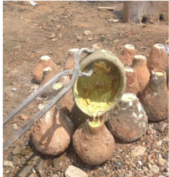
Figure 14. Molten brass poured into mould.
