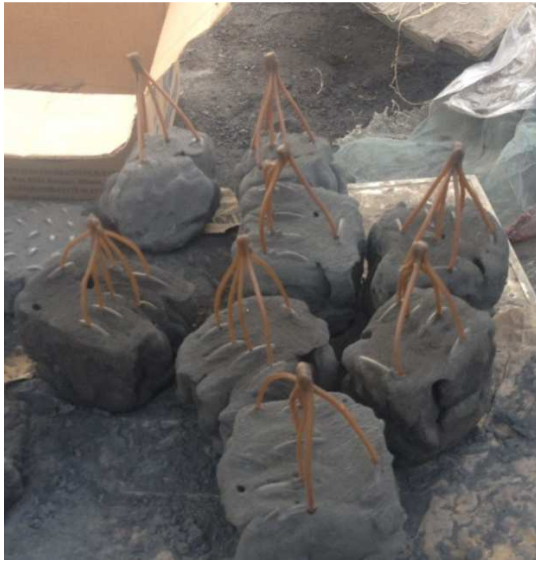
Figure 12. Wax channels joined together.
