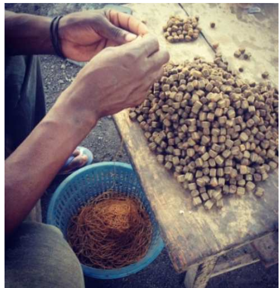
Figure 6. Wax threads for hollow cast design.
