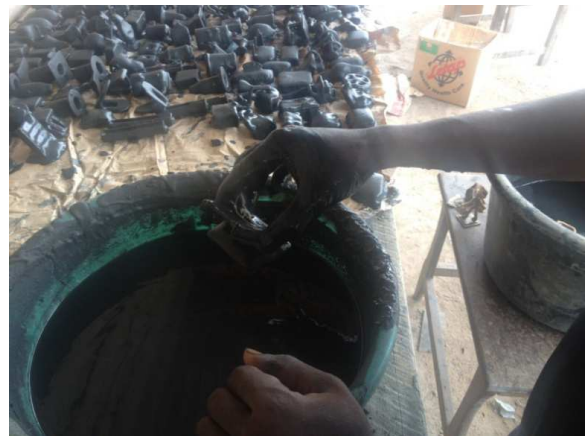
Figure 10. Coating wax models.
