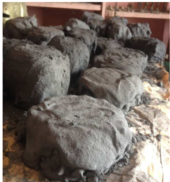
Figure 10. Coating wax models.
